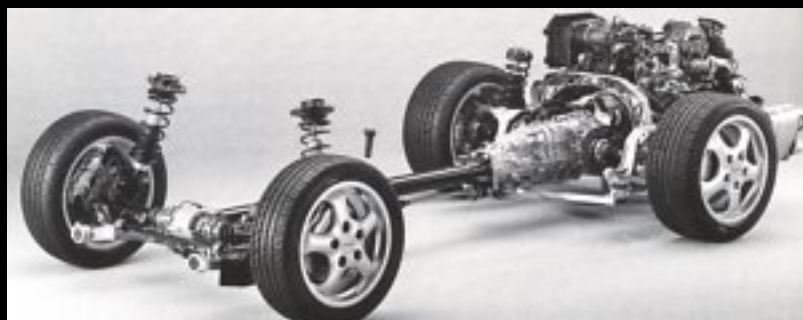
Left: 993's 4-wheel drive system; Right: a typical viscous-coupling differential
