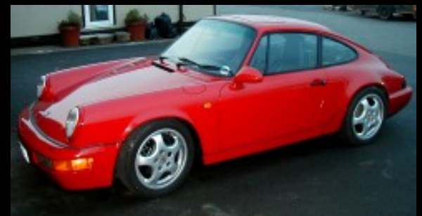
The ever popular 17" cup/turbo 1 style rims. Note that the RS used an extremely lightweight, forged version of these rims.
