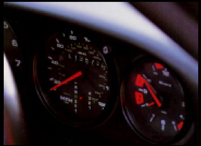
Tiptronic equipped cars had the details of gear engagement on the rev limiter.
