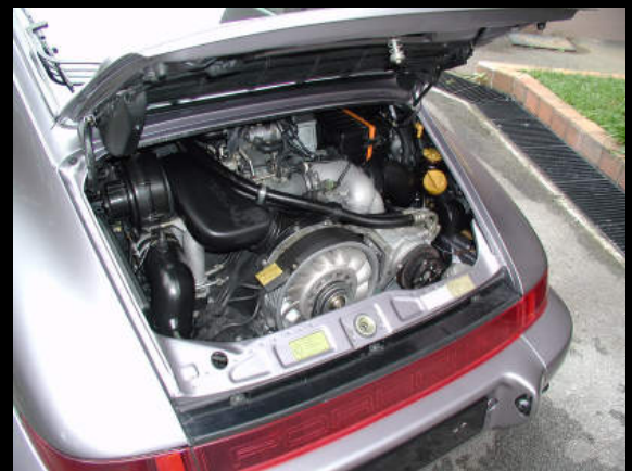
Above engine has Cup bypass pipe replacing the original primary muffler- a common upgrade.
