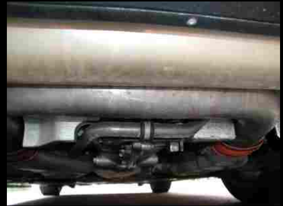
Rear engine pan with air duct whilst providing aerodynamics, can be removed for better engine cooling with little effect on aerodynamics.
