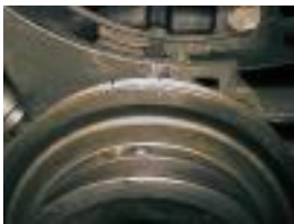
Figure 12: TDC 'Z1' Mark Aligned with Case Centerline
