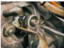
Figure 17: Adjusting Intake Valve with Feeler Gauge
