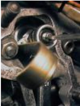
Figure 16: Tightening / Loosening Retaining Nut
