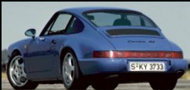
Rear spoiler rest at low speed ...
