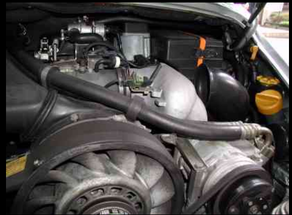
The 3.6 engine. Note that the air box can be updated to the 993 air box and air flow system for substantial power gains.
